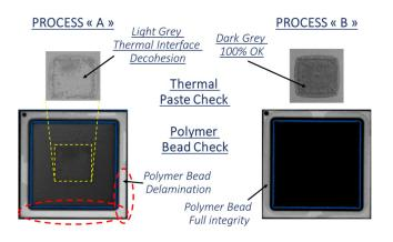
Fig. 7: Package assembly integrity check after Deballing / Reballing
