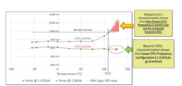
Fig. 5: CPU Frequency versus Supply voltage.
