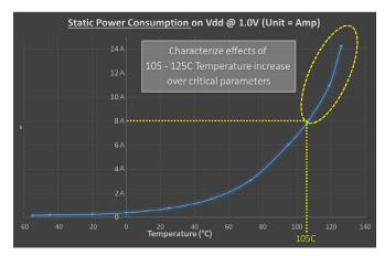
Fig. 4: Power Consumption versus Temperature.
