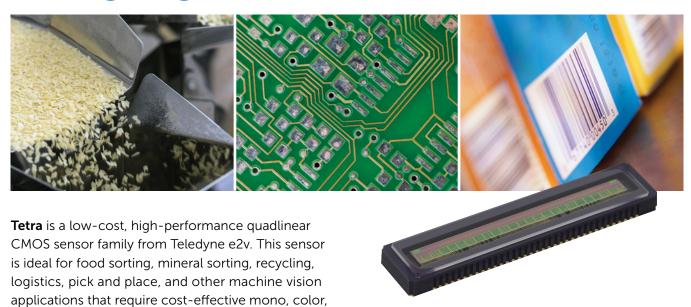
The monochrome sensor has a resolution of  $4,096 \times 4$  pixels with a  $7 \times 7$  µm pixel size and runs at a maximum line rate of 128 kHz aggregate. Based on a synchronized shutter design, the sensor provides low read noise and high dynamic range through the use of digital Correlated Double Sampling (CDS).
